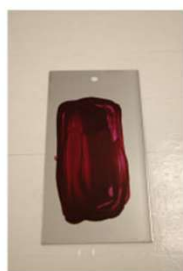
Stainless steel coupons are spiked with sample soils.
