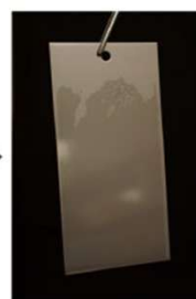
Coupons are evaluated: Visually clean? Water-break free? Weight change?
