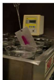
Coupons are exposed to multiple cleaning parameters depending on objectives.
